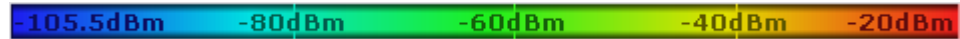
Fig. 6-6: Linear color curve shape = 0; colors are distributed evenly over the complete result range
